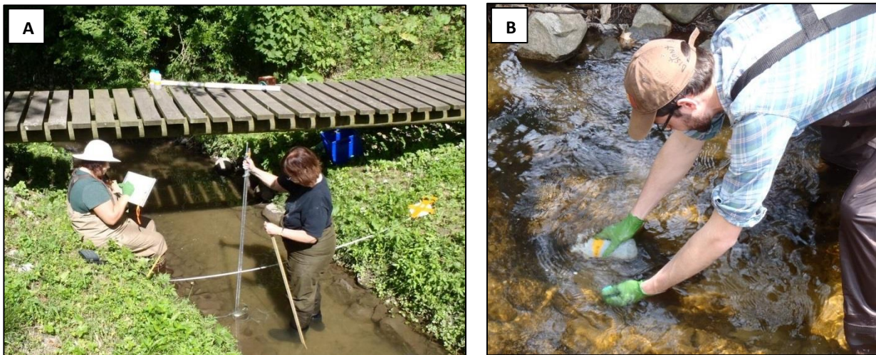
Figure 2.1: Researchers measuring streamflow (discharge) in Fremont Drain (A) and collecting water samples from Brooks Creek (B).
